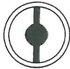
Gas Regulator shown in LP Gas position
